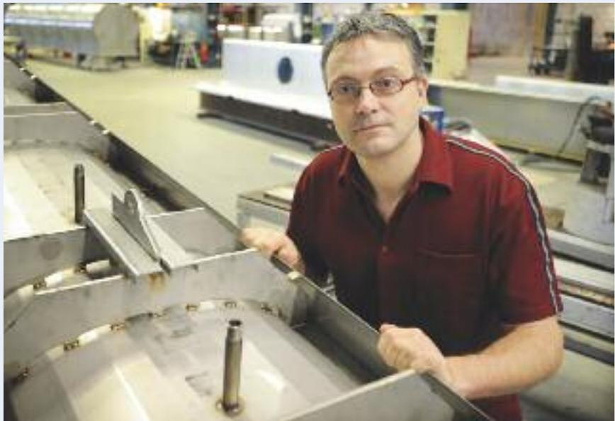
are hygienically designed; all contact parts are stainless steel and include a 'Cleaning in Place' system. This means they can be cleaned on location semi-automatically.'
