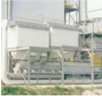
requires a separate cooler resulting in a 50–60% increase in the installation cost. A continuous fluid-bed dryer/cooler will always be smaller for a given throughput than a rotary drum installation.
