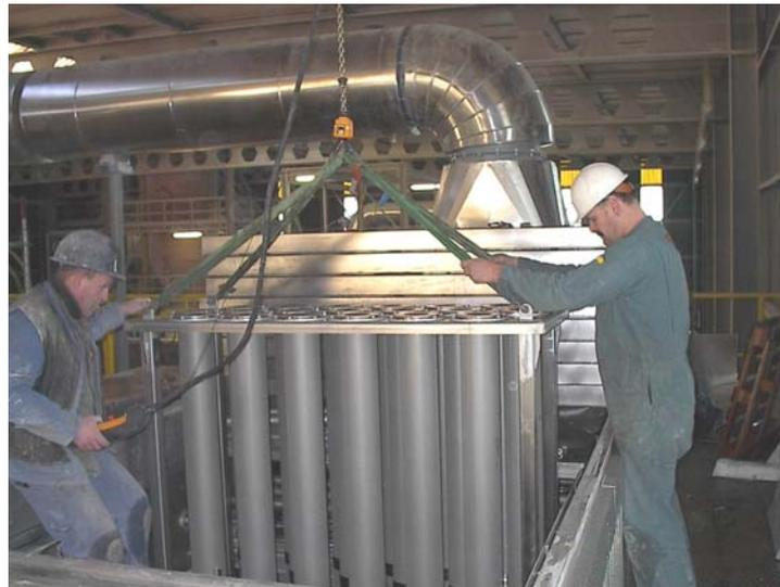
**JETBAG FILTER with stainless steel fibres filter elements**
