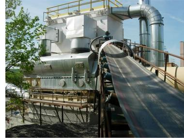
**VENTILEX FLUID BED DRYER FOR SAND & GRAVEL**
