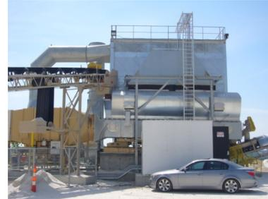
200 TPH VENTILEX Aggregate Dryer system in Missouri
