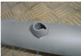
Image 2: Damaged blow-pipe nozzle from water in compressed air line
