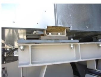
Serious damage to the dryer will occur if these bolts and washers (also known as sliders) are not adjusted to allow movement of the dryer during expansion and contraction. The area around the sliders must also be kept clear of debris.
