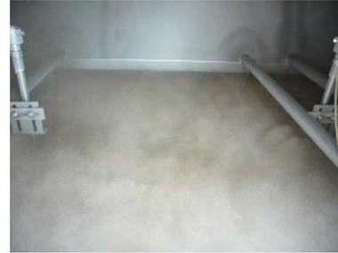
Fluidized sand inside of a VENTILEX Sand Dryer
