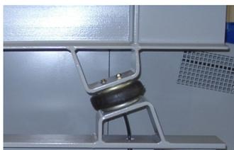
Air Bellows, or as some refer to them as Air Springs, are the little devices that provide the cushion for the VENTILEX Drive during the shaking motion while in operation. A clear advantage over the high frequency vibratory style of other fluid bed dryers, the shaking motion using the air bellows allows the VENTILEX Dryer to demonstrate true plug flow for your product (first in, first out), and allows for much less stress on the Dryer by keeping the frequencies low.
